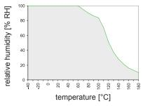
The grey area shows the allowed measurement range for the humidity sensor.
