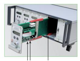
push-buttons for humidity / temperature calibration adapter PCB
